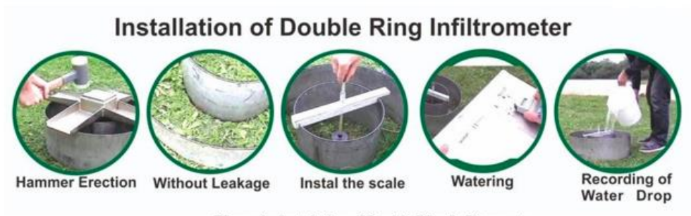
Figure 2: Instalation of Double Ring Infiltrpmetr
