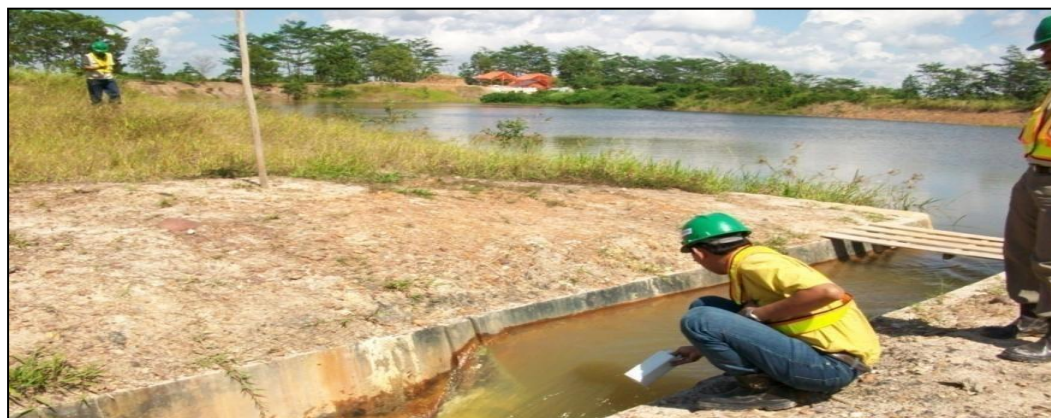
Gambar 6. Proses pengapuran KPL di pit 3 Barat Banko Bara Sumber: Sari et.al (2018)
