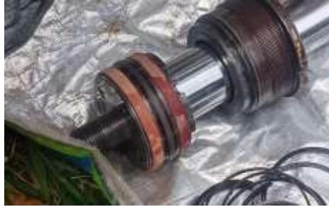
Figure 5. New wear seal on cylinder piston
