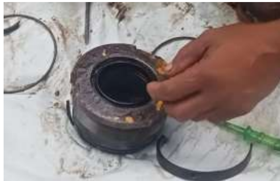
Figure 3. Dust seal removal
