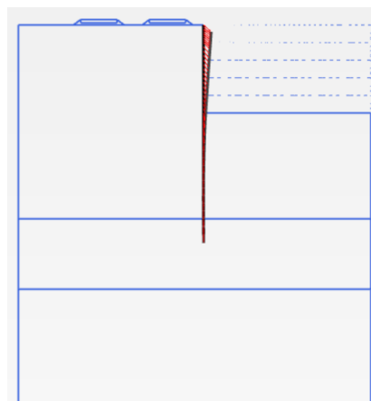
Gambar 6. Total displacement dinding galian
