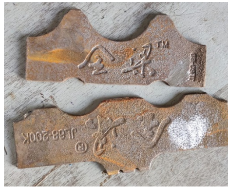
Figure 6. Horizontal and vertical anti-abrasion grid sample
