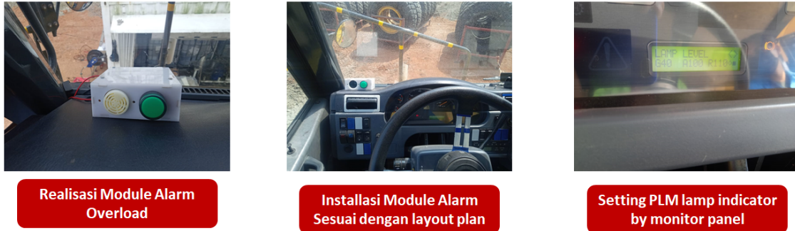
Gambar 3. Implementasi sistem Early Alarm Indicator
