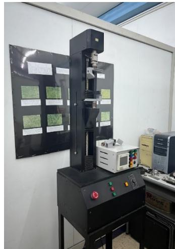
**Gambar 2. Alat uji *bending test***
