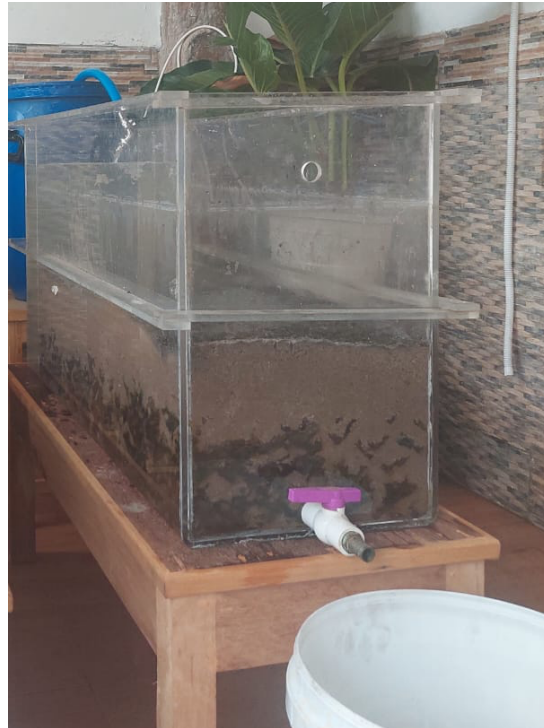
Figure 1. Reactor Constructed Wetlands Source: Author, 2024
