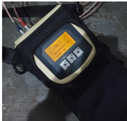
Gambar 1 Alat Ukur Ultrasonic Flow Meter
