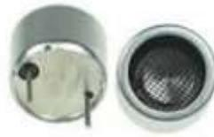
**Gambar 3. Sensor Ultrasonik**
