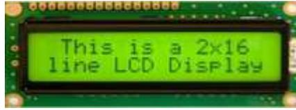
**Gambar 2. LCD 2x16**
