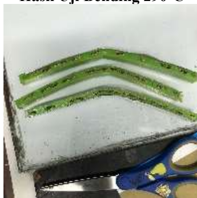
Gambar 22 Hasil Bending 300°C
