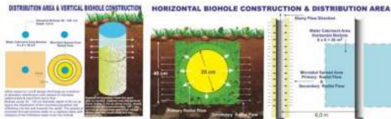
Gambar 2. Distributiom & Biohole Structure
